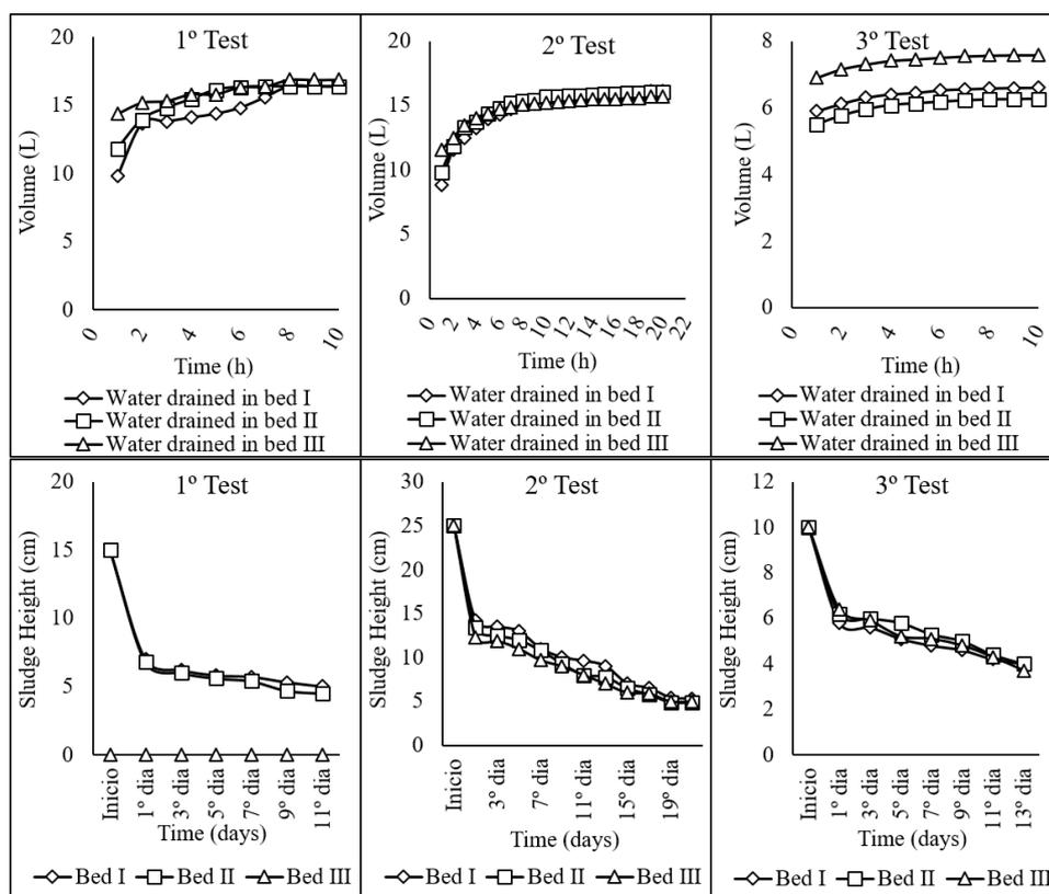
**Figura 1.3** – Free water drainage and sludge height variation in dewatering
