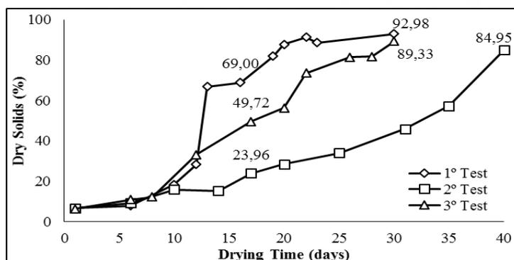
Figure 1.4 Average solids content of sludge
