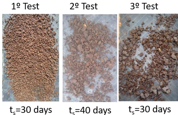
**Figure 1.5** Appearance of the sludge at the end of each test
